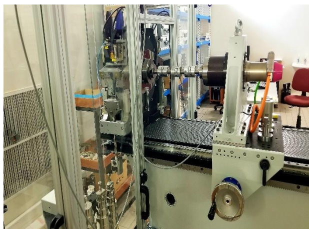
Calibration (set up) of a 50 N m static torque transducer, using the 50 N m Lever mass, torque standard machine (TSM-DW-50-Nm).
