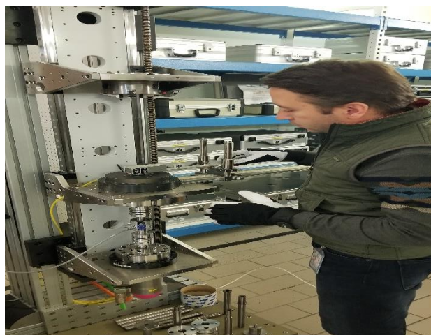
Calibration (set up) of a reference torque wrench using a static transducer installed onto the 100 Nm torque calibration machine (TCM-RTT-100-Nm).
