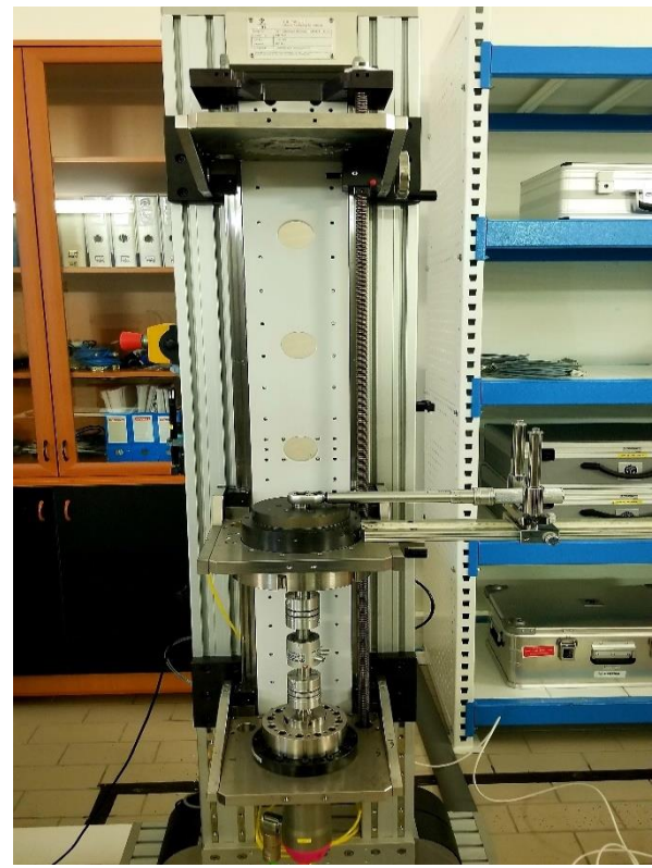
Calibration set up for type 2, class D (left) and type 2, class A (right) hand torque tools using the 100 N m Torque Calibration Machine (TCM-RTT-100-Nm).
