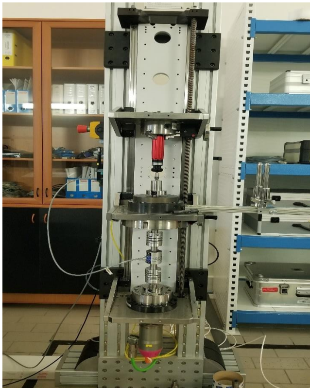
Calibration set up for type 2, class D (left) and type 2, class A (right) hand torque tools using the 100 N m Torque Calibration Machine (TCM-RTT-100-Nm).
