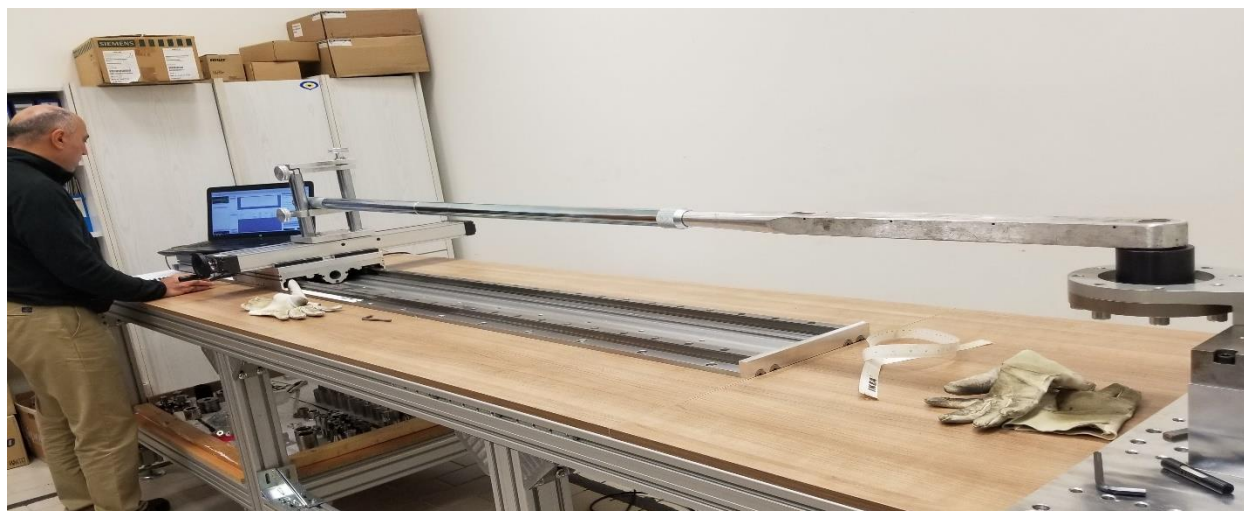
Calibration of a type 2, class A torque wrench (3000 N m) with arm length extension using the 3000 N m Hand torque tool calibration device (T-RTT-03).
